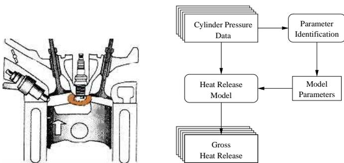
A thermodynamic model is necessary for data extraction.
