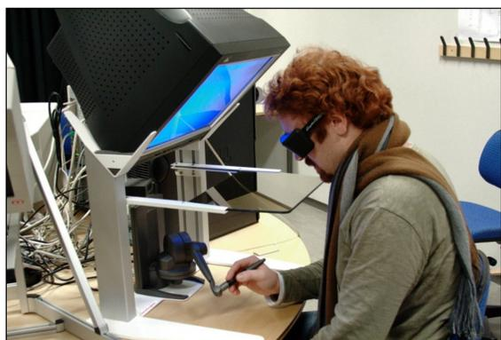
The application is running on a Sense-Graphics IW presenting active stereo 3D graphics and co-located haptics through a Desktop PHANToM.
